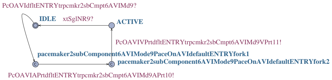
Figure 15: Translation of the AND superstate corresponding to the AVI mode. Merely the two substates AVI-A and AVI-V are activated.
